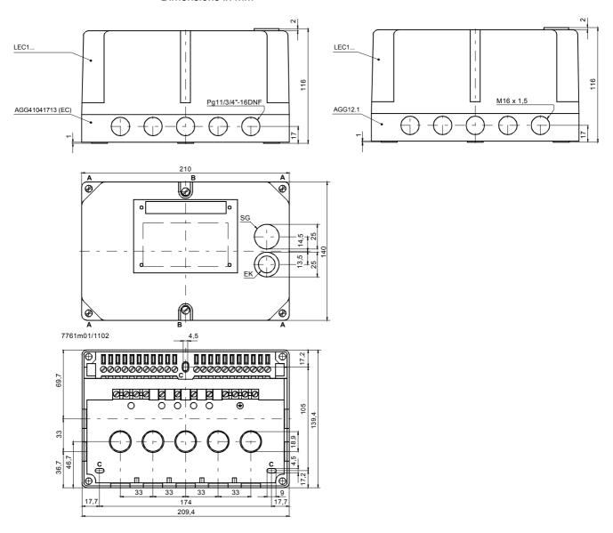
To remove the control unit from the plug-in base, loosen **only** the 4 screws  $\bf A$ . To remove the unit cover, also loosen the 2 screws  $\bf B$ .
