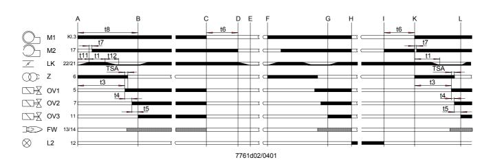
Double- or multiflame supervision of gas burners (expanding flame burners) Startup with short preignition (3 seconds) and checked actuator control. Required type of flame safeguards: LFE10... with UV detectors QRA... or ionization probe.
